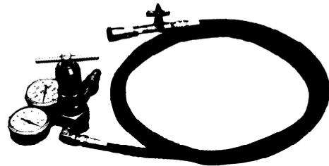
The NCA-1500 charging assembly is used to transfer nitrogen from a commercial bottle to the Super Nitro-Dyne system. The charging assembly includes a CGA-580 bottle fitting, regulator with bottle and system pressure gauges, shut-off valve, and 10 feet of high pressure hose with a fitting for the panel inlet.
